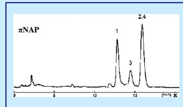
PYE column with its four-ring structure has enough  $\pi$ - $\pi$  interaction to resolve the peaks
