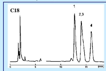
$\pi$ NAP column still does not have enough  $\pi$ - $\pi$  interaction to resolve the peaks
