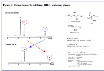
Figure 1 shows the separation of three polar compounds, neutral, basic and acidic, using two different HILIC stationary phases. The elution order of basic and acidic compounds was reversed between positively charged COSMOSIL HILIC stationary phase and negatively charged Atlantis HILIC stationary phase.
