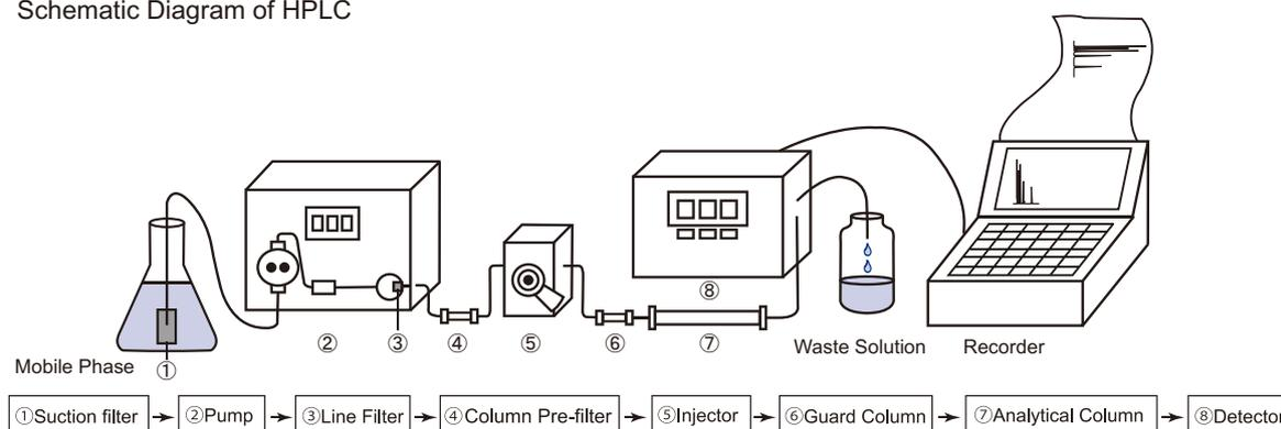
If elevated pressure is observed with the column disconnected, proceed to disconnect system components starting with the detector and moving backwards to the pump(s). If the pressure returns to normal, the component disconnected last can be identified as the problem.
