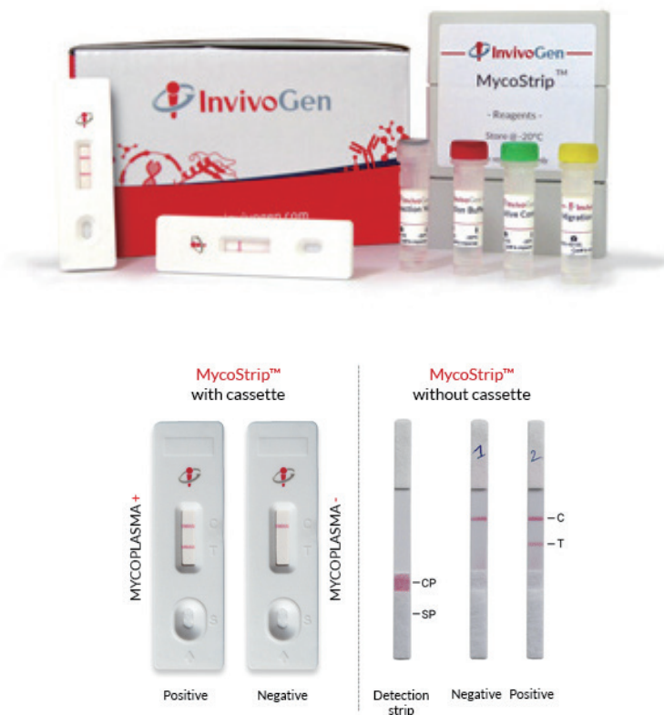
Figure 1. Mycoplasma detection using MycoStrip™ with or without cassette. SP: Sample Pad, CP: Conjugation Pad, C: Positive Control Band, T: Test Band.
