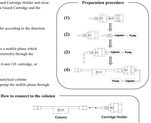
Column Connecting Tube Cartridge Holder
